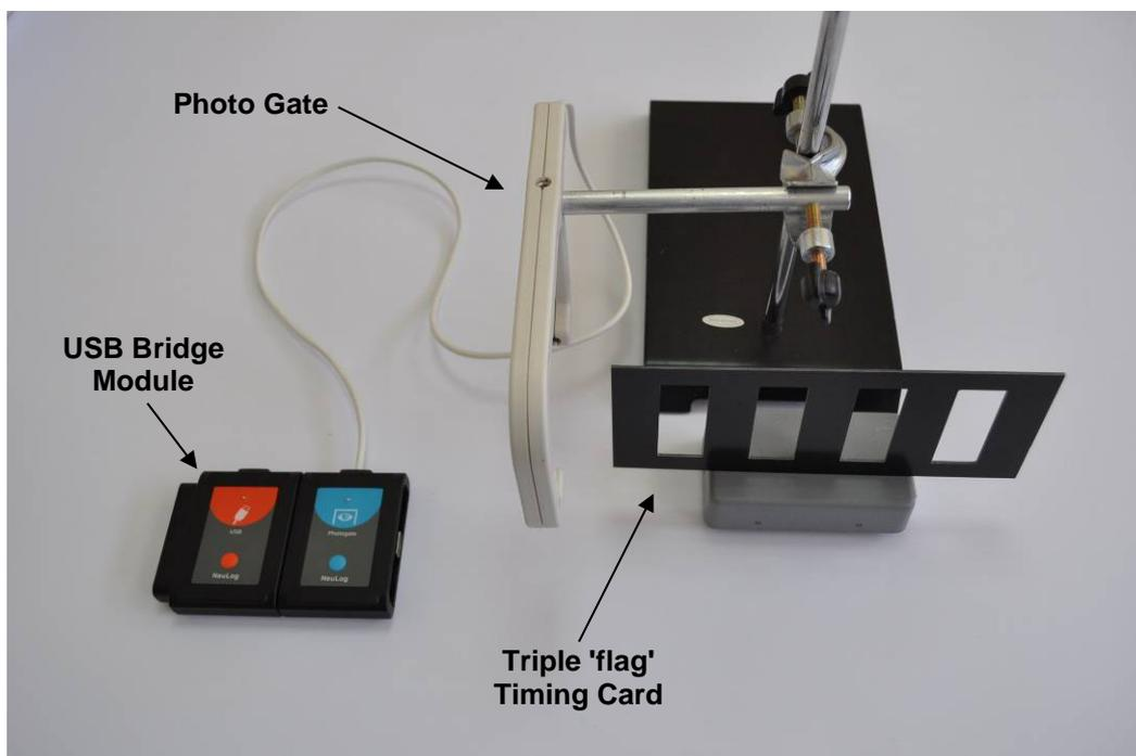
The apparatus setup required now is much like that used for the Time and Velocity mode and is shown in the photograph above.
