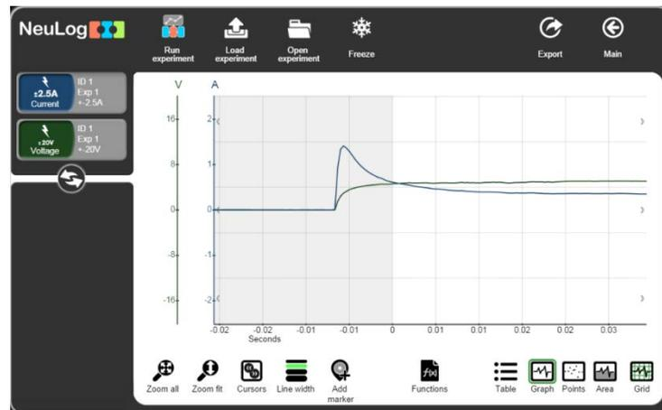
The interesting section of the above graphs is obviously just before the bulb was switched **ON** until the bulb was fully lit, where the two graph-lines level off. This section will be explained in more detail in the following page.
