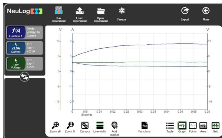
We can see how the resistance of the bulb goes up when the bulb turns on.
