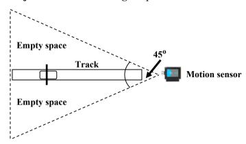
17. Ensure motion sensor **alignment** with the cart's path.
