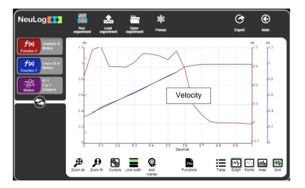
The velocity of the paper baking cup starts from zero, increases and then becomes constant.
