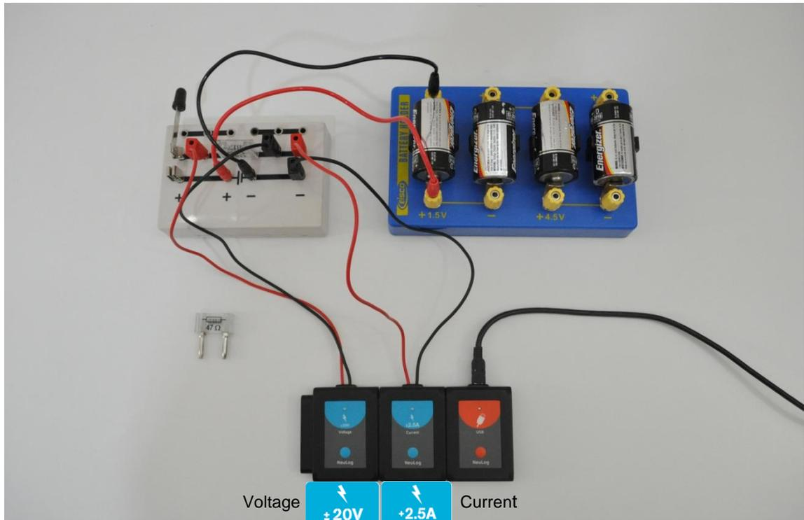
2. Connect the  $10\ \Omega$  resistor to the middle of the circuit board.
