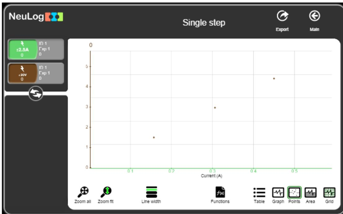
31. Click on the **Functions** icon
