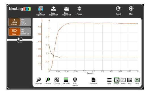
25. If the light measurement is saturated (it reaches the maximum sensitivity of the sensor) you can put the sensor at a greater distance from the bulb and repeat the measurement or you can change the sensors range.
