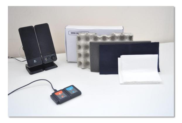
2. Put the sound sensor on the table in front of the sound source. Try to predict which materials will isolate sound better. Note that the sensor has an opening on the top through which sound is sensed.
