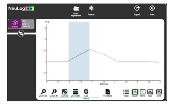
40. At this range, the cart moves away from the sensor (because of the slotted masses) and its velocity increases, therefore the acceleration is positive. The slope of the equation equals to the acceleration.
