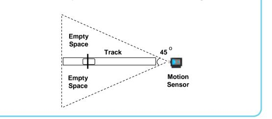
Make sure to remove any items located In the beam range.
