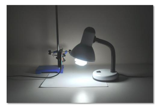
We are measuring light in the 0-6000 lx range because our maximal measured value is close to 1000 lx (you can change to the lower range if the intensity levels you get are lower than 700 lx).
