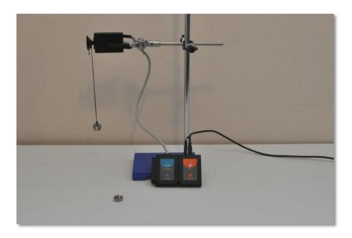
2. Tie one end of the thread to the 10 g mass and the other end to the rotary motion sensor. The length of the thread should be 25 cm (including the part between the thread and the rotary sensor axis) as in the picture below.
