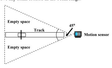
18. Ensure the motion sensor is correctly aligned with the cart's path.
