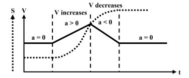
The velocity and distance of the cart can be described using the following equations:
