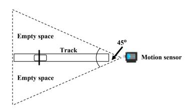
17. Before starting the experiment, ensure that the motion sensor is well aligned with the cart's path.
