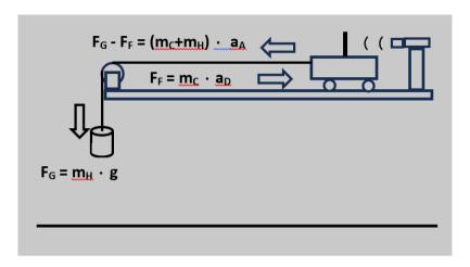
1. **Gravitational Force** ( $F_G$ ): The force pulling the cart is the weight of the hanger and its attached masses. We denote it as  $m_H$ .
