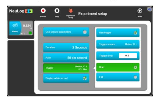
28. Bring the cart to a distance less than 30cm from the sensor and click on the **Record** button.
