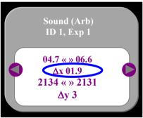
19. The time for one cycle (T) appears on the left of the screen. is 1.9 milli seconds = 0.0019 s.
