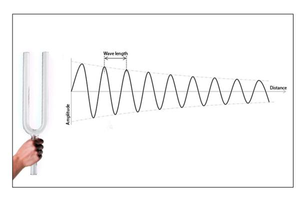
The image above illustrates the propagation of sound waves from a vibrating tuning fork. The waves diminish over distance (requiring close measurement) and over time (*necessitating quick data collection*).
