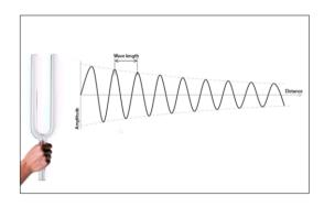
The image above illustrates how sound waves propagate from a vibrating tuning fork. The waves decay over distance; which is why measurements should be taken close to the tuning fork. They also decay over time, so measurements should start immediately after striking the fork.
