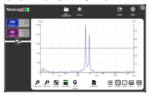
The FFT (Fast Fourier Transform) function displays the constituent frequencies and their amplitudes of the measured signal.
