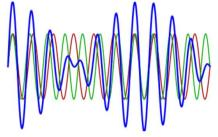
This experiment explores how two tuning forks with slightly different frequencies produce beats. The frequency difference between the two forks determines the **beat frequency**, a concept used in **tuning instruments and medical ultrasound applications**.
