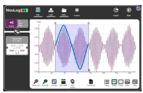
On the left you can see dx, the time difference between two cursors on the graph. In this experiment, dx = 50 milliseconds.
