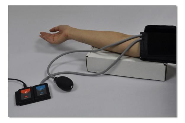
Wrap the cuff tightly, without causing discomfort, around your partner's upper arm. Ensure that the rubber tubing (connected directly to the blood pressure cuff) is situated a couple of centimeters above the inner elbow. The subject's arm should be supported and the cuff around it should be at the same level as the heart.
