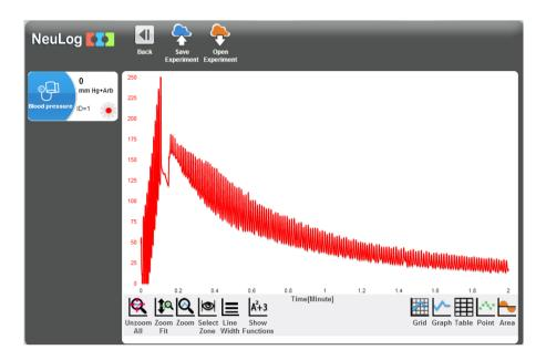
The pressure at the end of the measurement should be around 40 mm Hg. If the pressure did not go that low you have to either repeat the measurement, opening a little more the release valve or increasing the duration of the measurement to 3 minutes.
