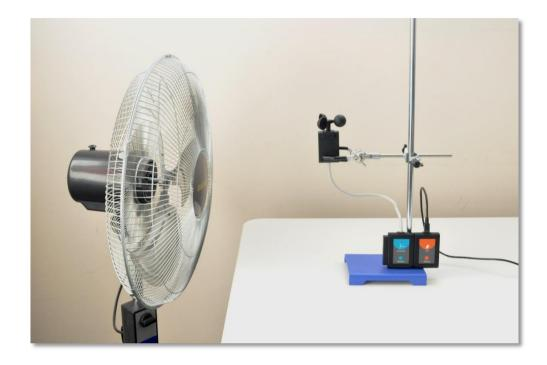
2. Place the fan on the table and the anemometer in front of it at a distance of approximately 30 cm.
