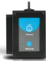
This transducer is built as a strain gauge with Wheatstone bridge circuit so its output is a voltage that depends on its absolute pressure.
