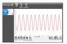
In dB mode, the wave is sampled and the average intensity (calculated by the sensor's controller) is converted into dB value.
