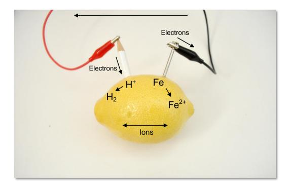
At the Fe electrode, Fe atoms are converted to  $Fe^{2+}$  ions which are released to the lemon. The electrons flow to the C electrode (through the cables) where hydrogen (H<sup>+</sup>) ions from the lemon's acid are reduced to H<sub>2</sub> gas. The carbon electrode conducts the electrons and does not participate in the actual reaction. Positive and negative
