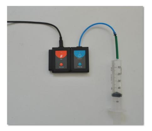
2. Pull the syringe's plunger up to the 50 ml position and tightly connect the syringe to the sensor using the adaptor tube.
