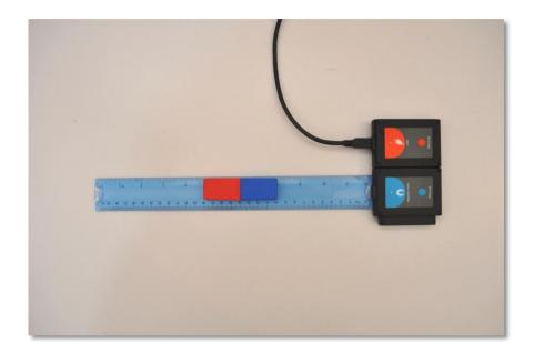
Place the magnet (with the plastic case) on the ruler. The blue south pole of the magnet should be directed toward the sensor and the magnet's edge should be 14 cm from the sensor.
