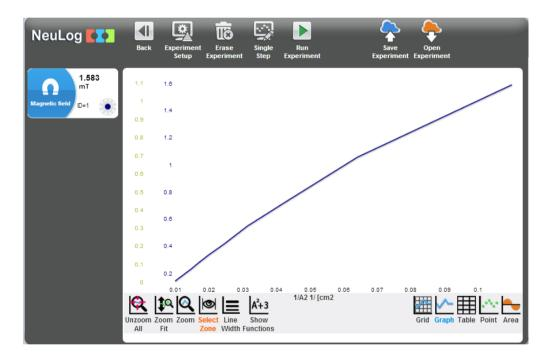
25. We can see that we get a linear relationship between the magnetic field strength and the inverse square of the distance from the magnet.
