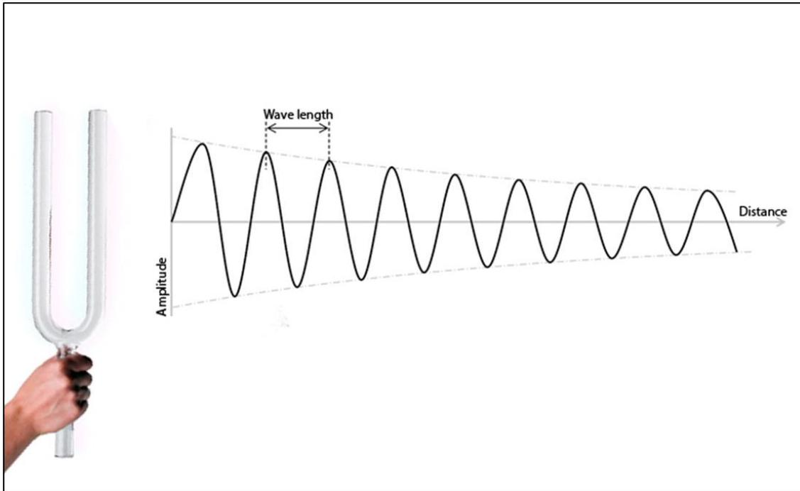
The image describes the way sound waves are propagated by the tuning fork motion. The waves decay over distance; therefore we should measure them close to the tuning fork. They also decay over time so the measurement should be started right after hitting it.
