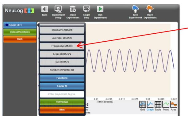
34. Repeat this procedure with the other tuning fork and write the measured frequency in the table on section 23.
