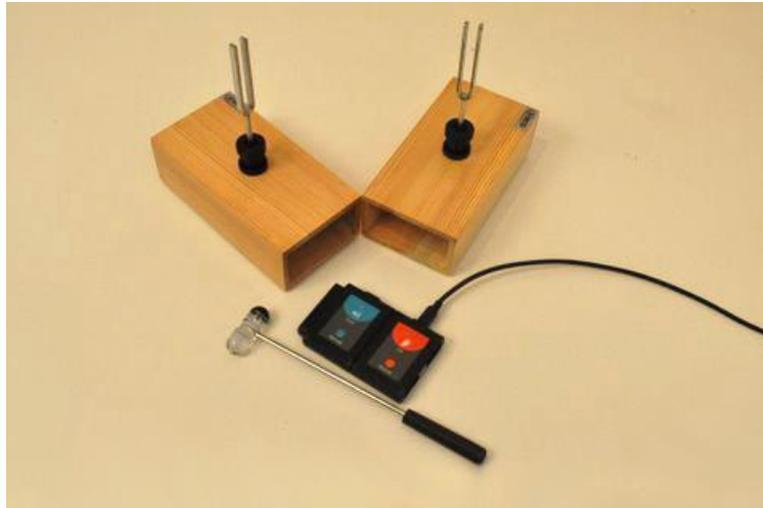
2. Introduce the 480 Hz tuning fork in one of the resonance boxes and the 512 Hz tuning fork in the second.
