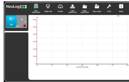
6. Once a sensor module box appears on the left side of the screen, the sensor will give a live reading in its module box and on the graph appearing on the screen and you can begin experimentation.
