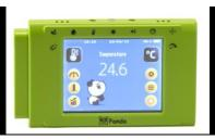
NeuLog Panda can work with external sensors (up to 5 at a time) as well (these are not included in the Panda package).
