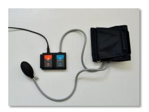
The three ranges of the sensor show the real measured pressure (in mm Hg.), only the pressure amplified fluctuations (Arb), and the combined signal of both of them.
