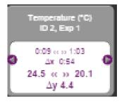
22. Look at the data at the bottom of the graph, we can see that the temperature dropped from 24.5 °C to 20.1 °C in the sample measurement.
