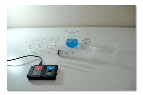
2. Make sure you have 80 ml of a food coloring solution with an absorbance of 1-1.5 in a 250 ml beaker. Mark the beaker as "100%".
