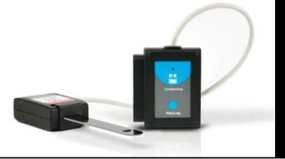
of ions present in a solution the easier an electrical current can flow and a higher conductivity value will be measured.
