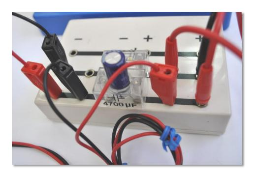
8. Make sure the capacitor's + side is near the red cable of the voltage sensor.
