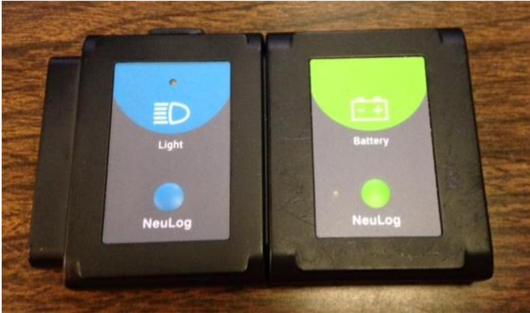
To start the data collection, press the blue button on the sensor. While data is being collected, the red light on the sensor will be lit.
