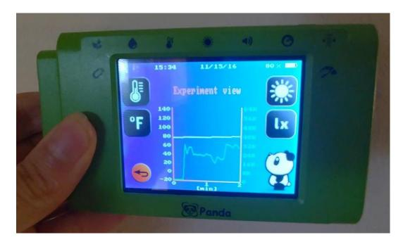
18. We can see that after turning on the lamp, light intensity immediately increased. Fluctuations in the light measurements can occur because of slight movements of the hand during the measurement. The temperature also increased a bit, but that change is a lot slower.
