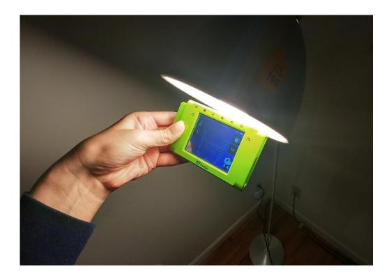
If you are using an incandescent light bulb you should place the Panda a few inches from the bulb and make sure it does not get too much heat, or you can also conduct a shorter experiment. Be careful not to touch the light bulb with your hand.
