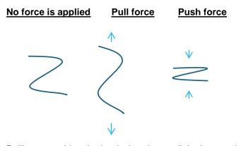
Pulling or pushing the hooks bends very little the metal rod, changes the strain gauge resistances and the amplifier output voltage. This voltage is converted into force (N) by the sensor's controller.
