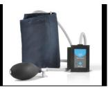
The pressure is converted into an electrical signal which separates into DC (mm Hg) and AC (Arb.) signals. The AC signal is amplified and added back to the DC signal to create the mm Hg + Arb. signal.
