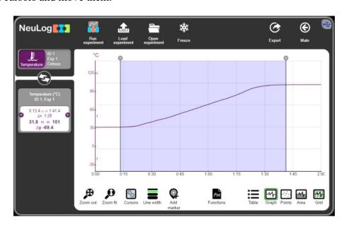
16. The measurement starts at room temperature and stops rising at 100 °C.
